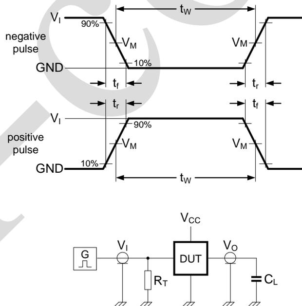
Figure 4. Test circuit for measuring switching times
